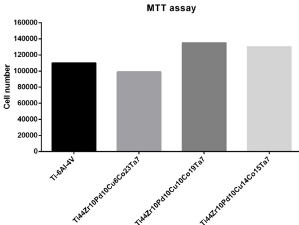
Figure 1. MTT assay of SaOS2 cells on Ti-6Al-4V and the series of novel Ti-based MG thin film.
